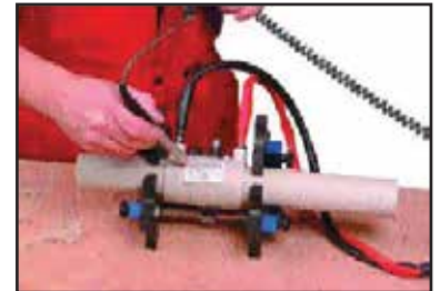
Scanning the bar code with a light pen
