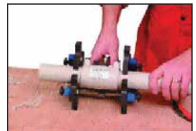
Once cooled, the joint can be removed
