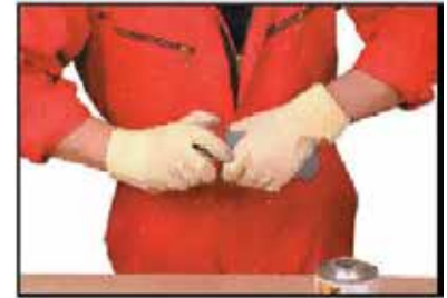
Chamfering the pipe
