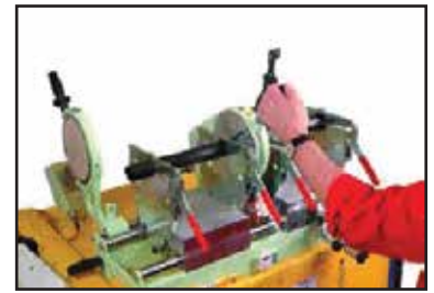
Planning the pipe
