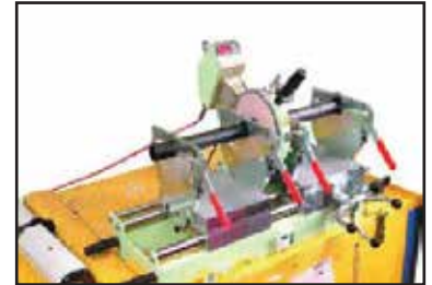
Heating of the pipes
