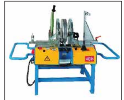
Butt fusion tool with hydraulic operation
