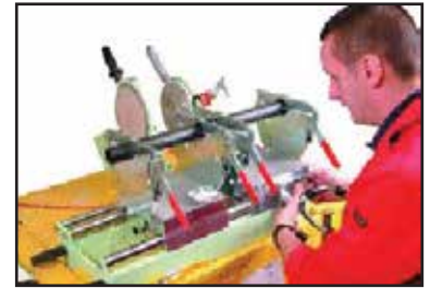
The heating element is removed and the pipes brought together
