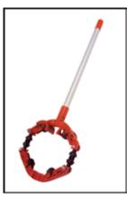
Pipe in diameters above 8"/200mm may be cut with large diameter wheel pipe cutters fitted with blades for use on plastic pipe. The cutters are fitted with outboard rollers to ensure that the cut remains square.
