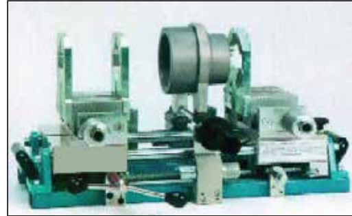
Bench socket fusion tool suitable for workshop or site
