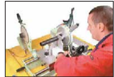
Peeling the pipe
