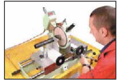
Heating the pipe and fitting
