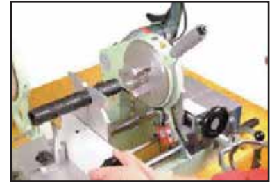
Preparing to peel the pipe
