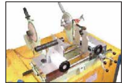
The fitting is mounted in the fusion machine
